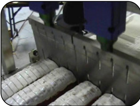
Ultrasonic Vibrations make Fast Clean Cuts
