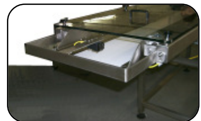
Tight nose discharge with Sensor for reciprocating control, Protective guard and Lexan Cover
