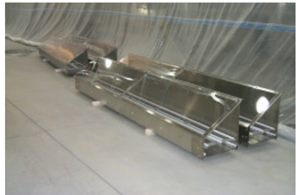
Conveyor frames with Lexan covers
